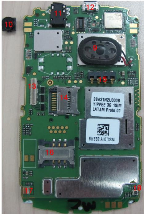
9. Speaker    10. Camera    11. Audio Jack    12. USB connector    13. FPC ZIF connector
